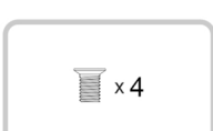
4 x M3*4 Flat Head Screw for 2.5" SSD (2 x Screw for Spare Parts)
